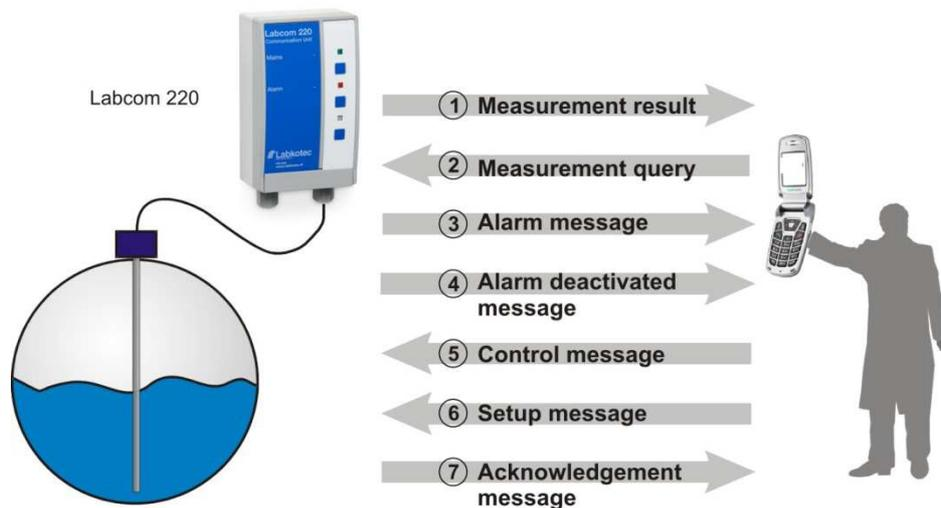
Figure 2. Message exchange between end users and Labcom 220
