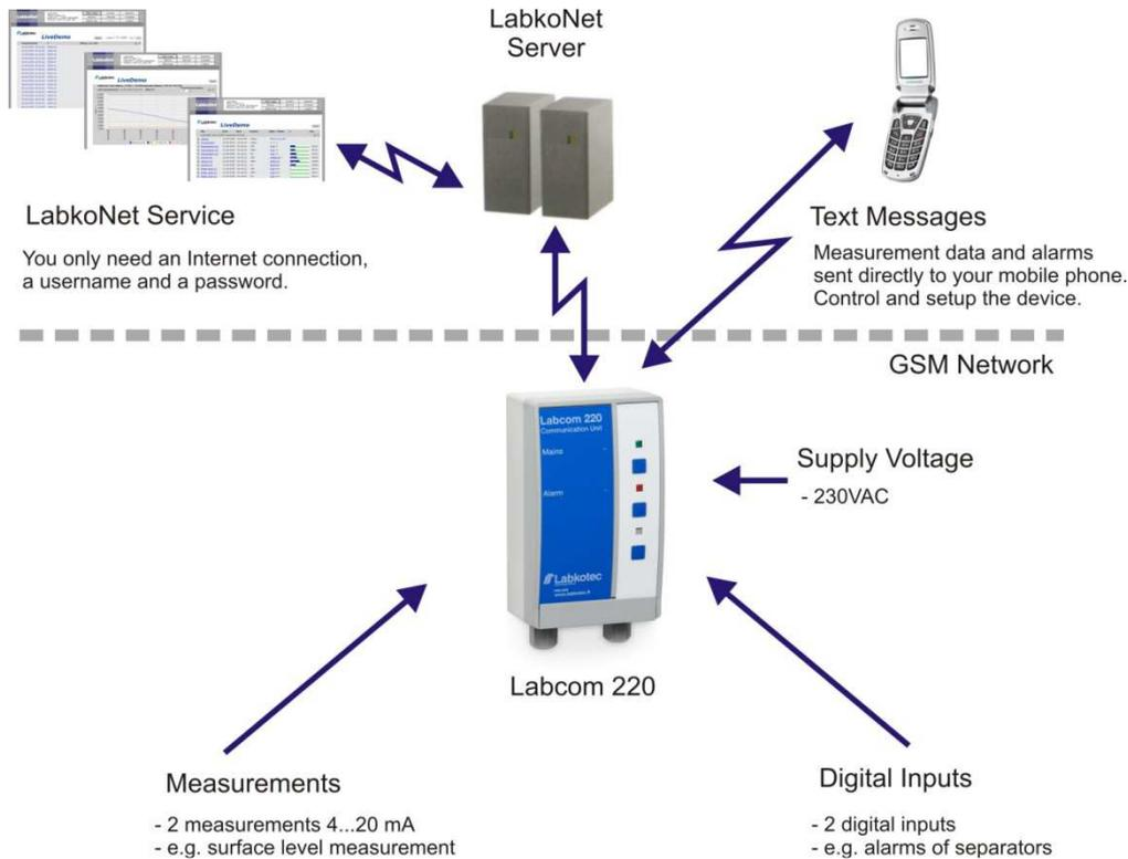
Figure 1. Labcom 220 interfaces to various systems
